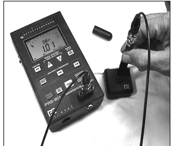
**Figure 6: Insert PRF-922 Fixture into PRV-913 Verifier and Measure Verifier Resistance**
