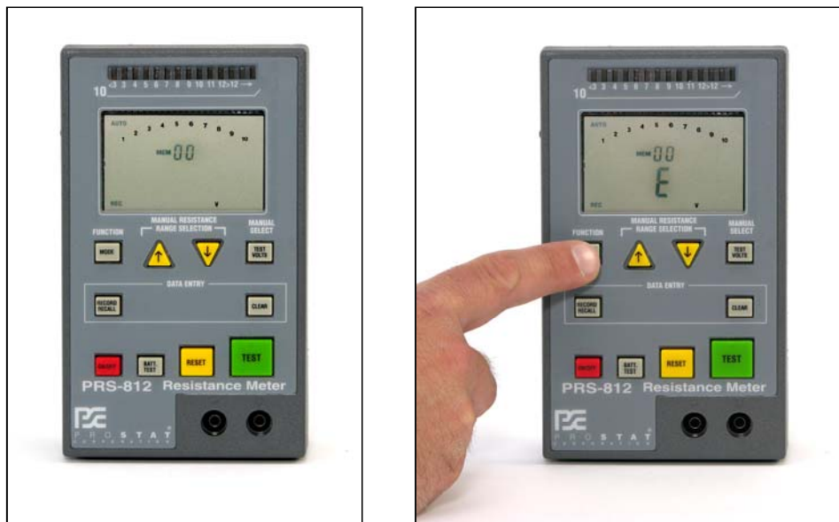
Figure 9: PRS-812 Powered Up in AUTO Exponential Mode (Right). To change to Ohms Data Display Press Function Mode button once. (Left)
