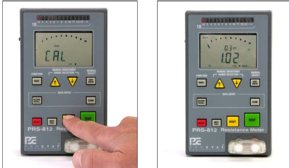
Figure 7: Complete Calibration Sequence by Pressing RESET. To confirm Calibration, Press TEST to measure the Calibration Shunt resistance. Shunt resistance should display 1.02 Ohms \pm 0.02 Ohms
