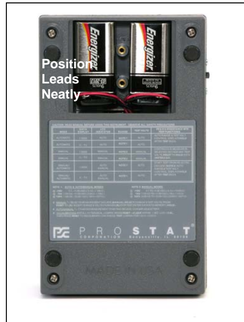
Figure 4: Install 2 each 9V Batteries
