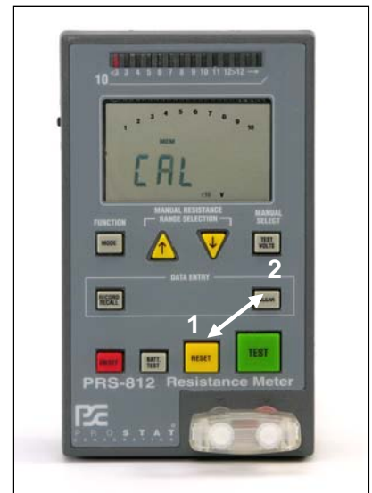
Figure 6: Start the Calibration Sequence by Pressing RESET then CLEAR within ½ Second
