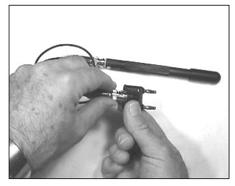
Figure 3: Connect Cable to Banana Converter
