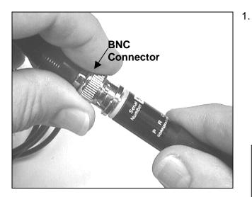
Figure 2: Connect shielded cable to PRF-922B's BNC fixture
