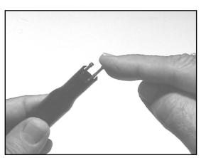
Figure 13: Insert Test Probe into its Socket and Press Firmly to fully seat
