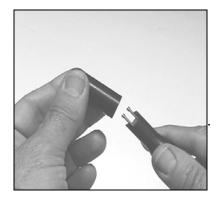
1. Connect the BNC/banana adapter to the wide range. resistance measurement instrument. Flange side of dual banana should be connected to the Positive (+) power terminal. This applies test voltage to the 10 outer ring electrodes.
