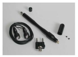
center-to-center. The electronic quality gold plated contact probes are 0.1-inch (2.54mm) in diameter, and are supplied with conductive synthetic rubber contact boots, which are 0.125-inch (3.18mm) diameter. The conductive boots are used to reduce contact resistance between the gold contact probes and materials under test in certain applications.
