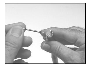
Figure 12: View of PRF-922B Spring-Loaded Test Pins and Socket
