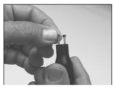
Figure 14: Installing Conductive Rubber Electrode "Boots"
