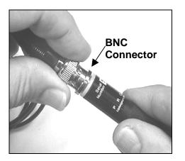
Figure 5: Connect shielded cable to PRF-912B's BNC fixture
