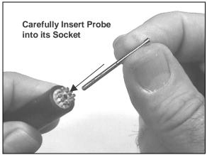
Figure 16: Insert Test Probe into its Socket and Press Firmly to fully seat
