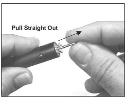
Figure 14: Remove Spring-Loaded probe electrode by grasping firmly and pulling straight out of its socket.
