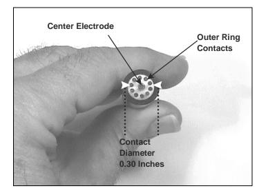
Figure 2: Concentric Ring Configuration
