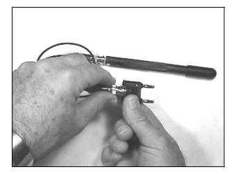
Figure 6: Connect Cable to Banana Converter
