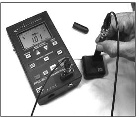
Figure 9: Insert PRF-912B Fixture into PRV-913B Verifier and Measure Verifier Resistance
