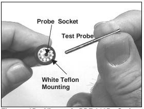
Figure 15: View of PRF-912B Spring-Loaded Test Pins, Socket & Teflon Mounting Disk
