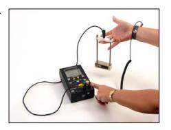
9. Clean the electrode with isopropyl alcohol prior to performing additional tests.
