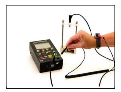
5. Balance the CAFÉ fixture electrode on the fingerprint side of the finger or thumb chosen in step 1 above.
