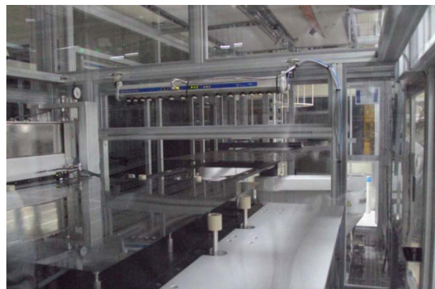
Figure 6. Conventional CDA ionizers in FPD process areas
