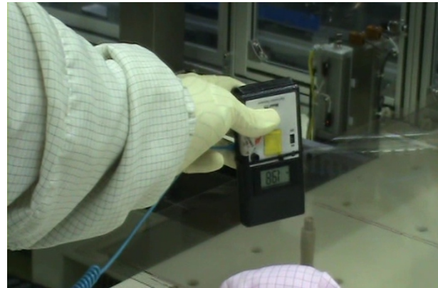
Figure 5. Glass charge detected at 1.98kV when separated from stage by lift pin
