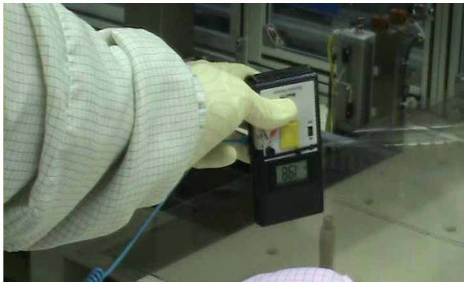
Typical Static Charge on FPD Glass Plate
