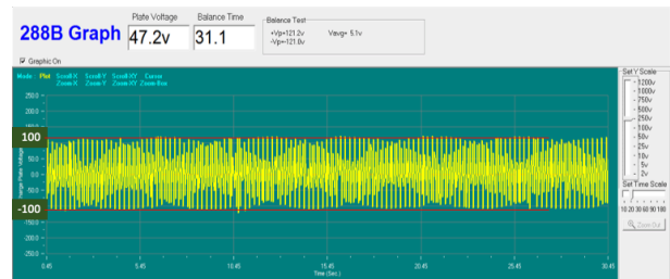
Figure 7: Model 288 CPM measurement result with 30Hz output of enhanced AC air assist bar ionizer.
