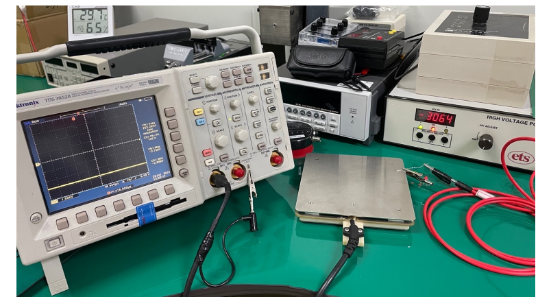
Figure 6 - CPM Plate to Oscilloscope and DC high voltage source
