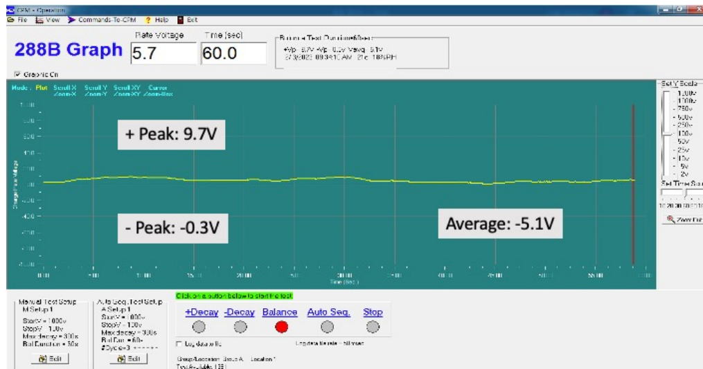
Figure 9 - DC Ionizer Test Results at 12-inch distance
