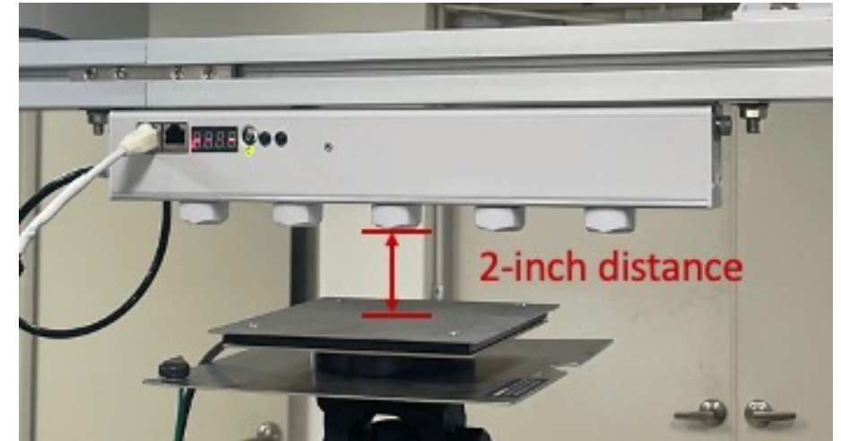
Figure 17 - DC Ionizer at 2-inch distance
