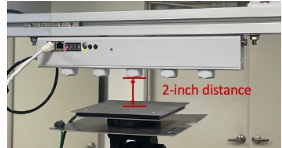
Figure 8 - DC Ionizer at 2-inch distance
