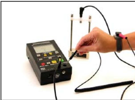
**Figure 3: Attach Wrist Strap cord to meter**
