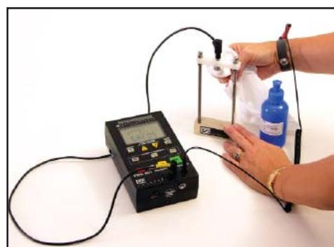
**Figure 6: Clean electrode with alcohol**
