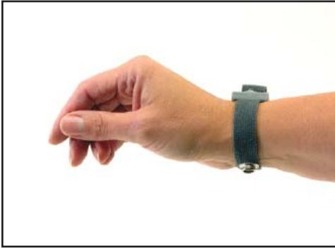
**Figure 1: Attach Wrist Strap to test hand**
