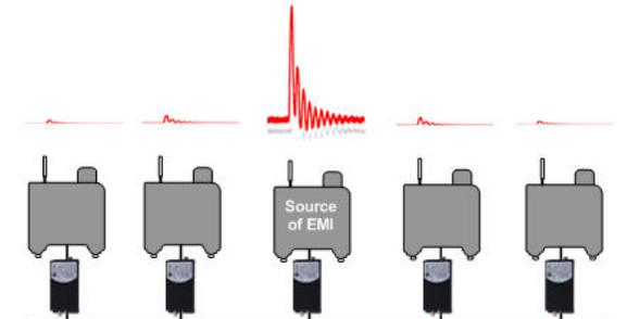
Figure 3. Ground filters GLE30-1 block propagation of EMI
