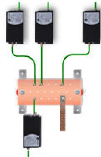
Figure 6. Connection of ground line filters GLE30 to a ground bar
