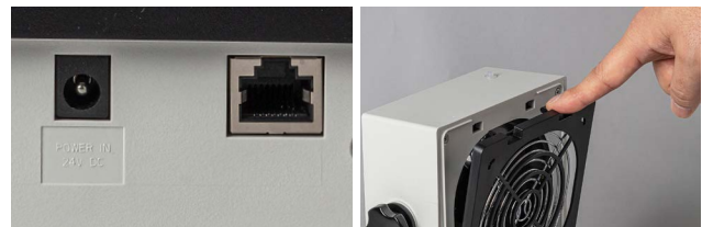
FMS monitoring through RJ-45 port
