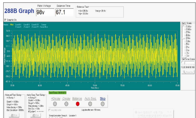
Induction Field Swing Voltage from Pulsed AC Ionizer Peak-to-Peak value: +305 V to -393 V
