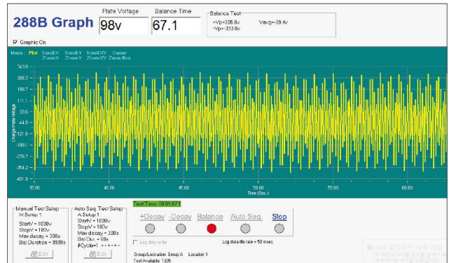
Induction Field Swing Voltage from Pulsed AC Ionizer Peak-to-Peak value: +305V to -393V
