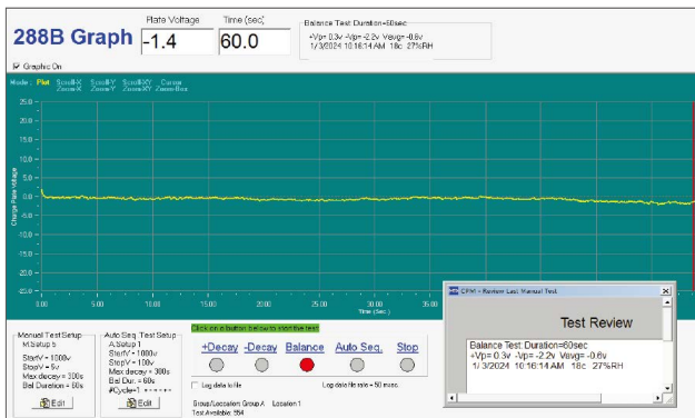
No Swing Voltage from Steady-State DC Ionizer
