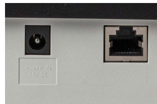
FMS monitoring through RJ-45 port
