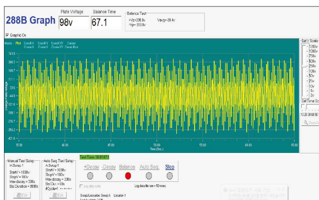
Induction Field Swing Voltage from Pulsed AC Ionizer Peak-to-Peak value: +305V to -393V
